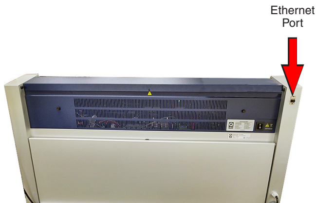
Figure 14.1: Ethernet port located on right rear of tester frame.
