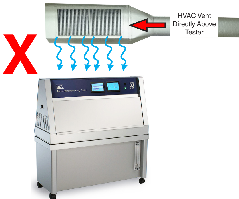
Figure 4.2d: Keep tester away from sources of hot or cold air.
