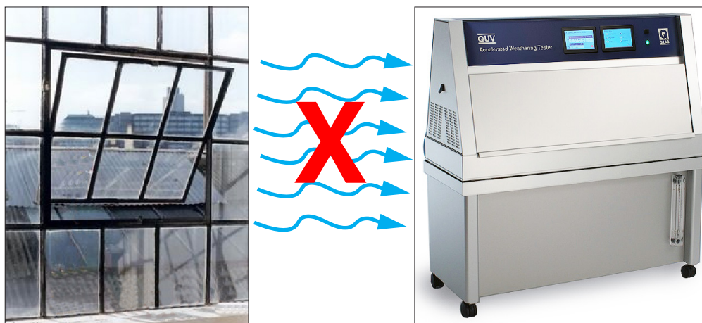
Figure 4.2c: Do not locate the QUV near open windows.
