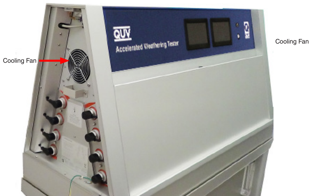
Figure 8.3: QUV left end cover removed showing cooling fan. Identical fan located at right end.
