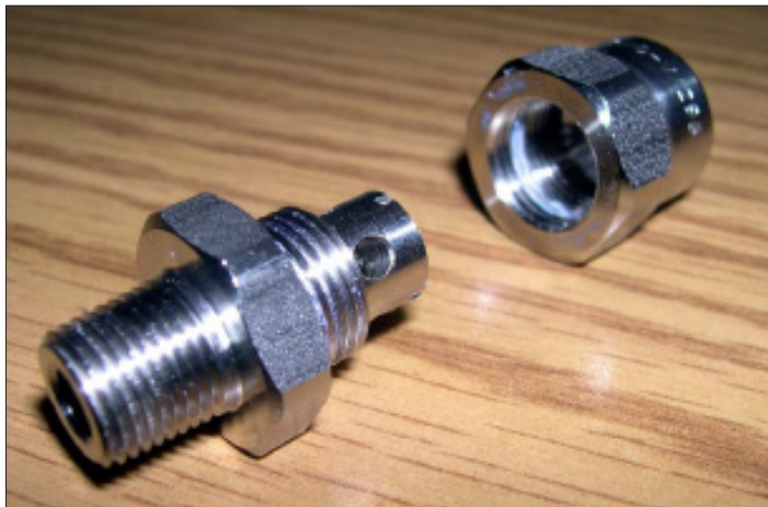
Figure 16.3b: Spray nozzle disassembled for cleaning.
