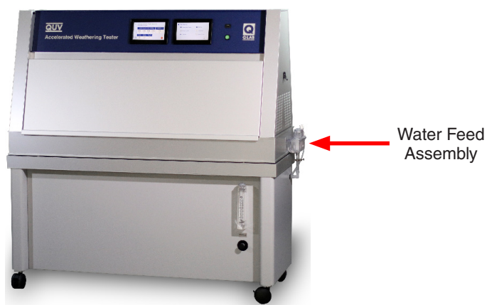
Figure 6.4a: QUV water supply connection location.
