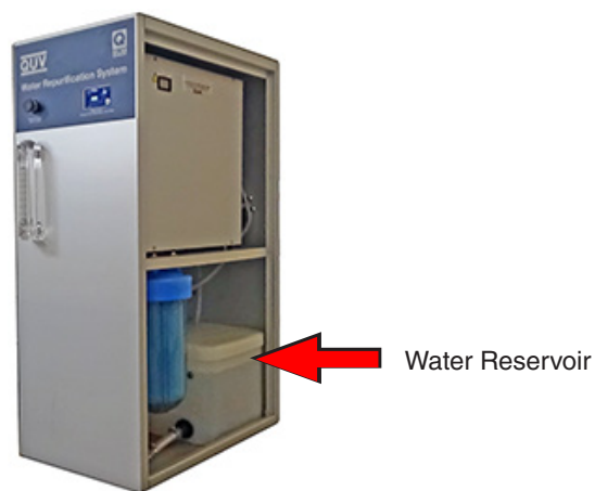
Figure 16.5f: Stand-alone water repurification system.
