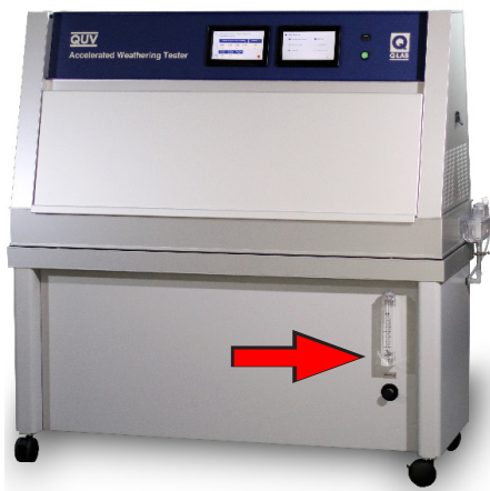
Figure 15.3b: Flow adjustment valve and flow meter location.
