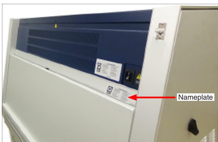
Figure 6.3: QUV rear view: nameplate location.
