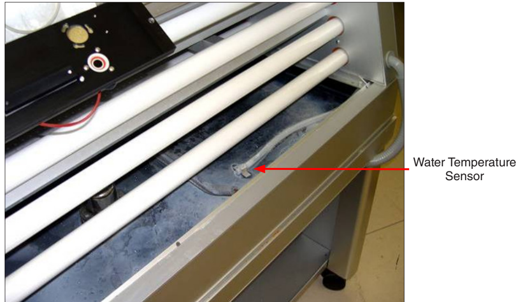
Figure 10.3: Water temperature sensor location (shown with water pan cover removed).
